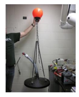
Figure 2. Methane bubble collector
